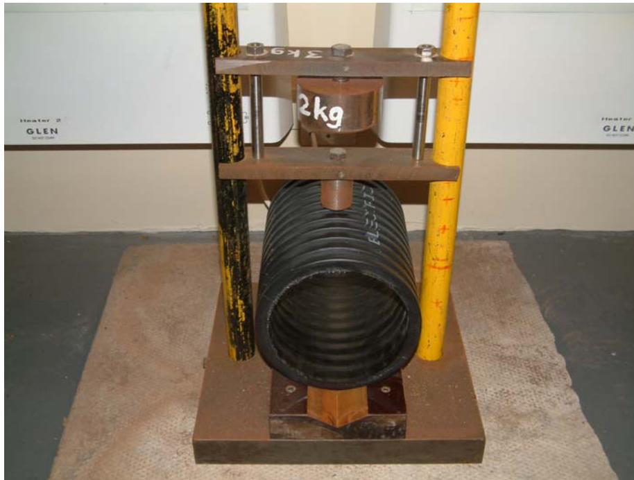
Figure 1 Impact test rig
