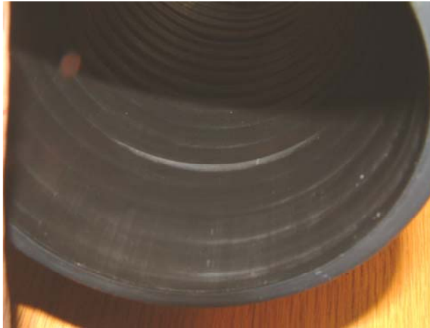
Figure 1 Defect on inside surface of 100mm duct
